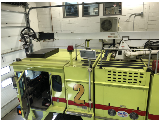
Photo 5: Engine 2 with High Reach Roof Turret
