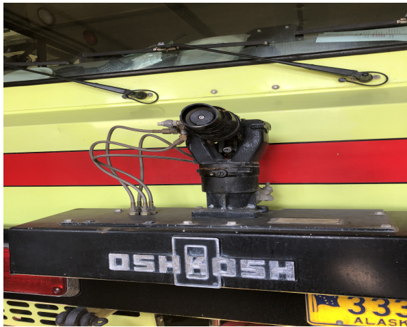
Photo 3: Engine 2 Bumper Turret
